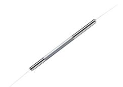
The FC Series 980/1550 nm WDM is based on Agiltron's advanced fused biconical taper technology and compact packaging structure. It features low insertion loss, high isolation, flat passband, high reliability, and stability. The device is ideal for 980 pump and 1550 nm signal wavelength division multiplexing in fiber optic amplifier systems.
